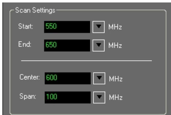
The most important parameters are the Start and End frequencies, which are set here. The Start and End frequencies can be set explicitly or implicitly, if you prefer, by setting the Center frequency and the Span. They are always specified in units of megahertz (MHz). Supported frequencies are 500 KHz through 4400 MHz.
