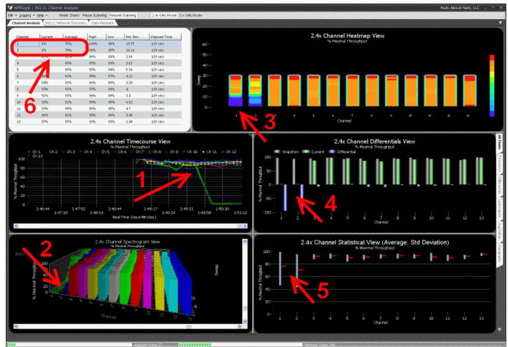
1. The Channel Timecourse view is useful for monitoring 802.11 channels as a function of time. Each channel is represented by a different line -- the x-axis is time and the y-axis is % Maximal Throughput. In this way one can clearly follow how RF interference affects different channels over time.
