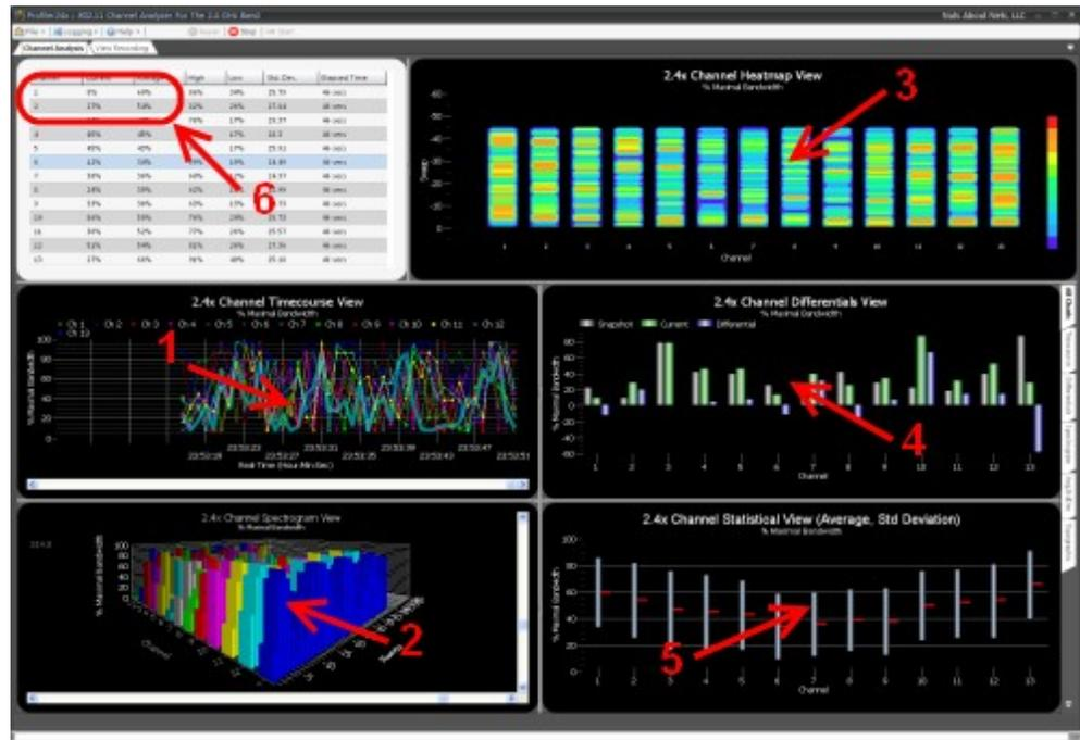
1. The Channel Timecourse view is useful for monitoring 802.11 channels as a function of time. Each channel is represented by a different line -- the x-axis is time and the y-axis is % Maximal Bandwidth. In this way one can clearly follow how RF interference affects different channels over time.
