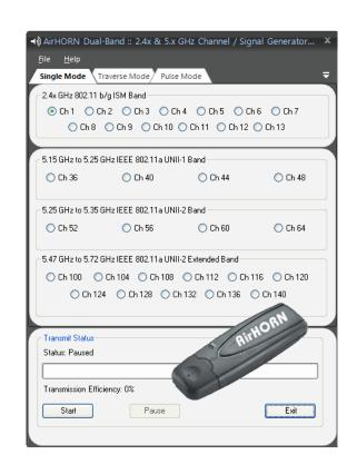
AirHORN is a unique, PC-based product that aids in testing Wi-Fi antennas, RF shields and wireless networks. It is an RF signal generator that covers the 2.4x and 5.x GHz ISM bands and was designed for microwave and RF applications.
